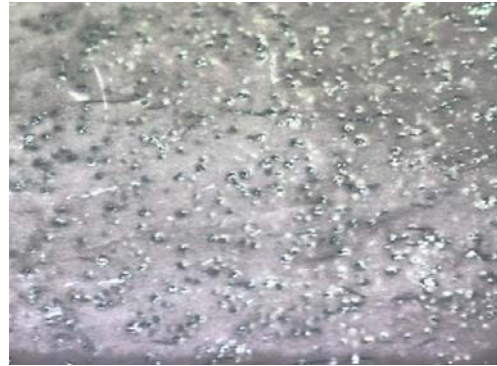
Figure 8b: PTFE/CaF 2 bearing 5µm wear loss
